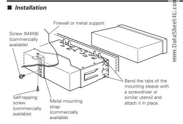
Make sure that the unit is installed securely in place. If the unit is unstable, it may malfunction (eg, the sound may skip).
